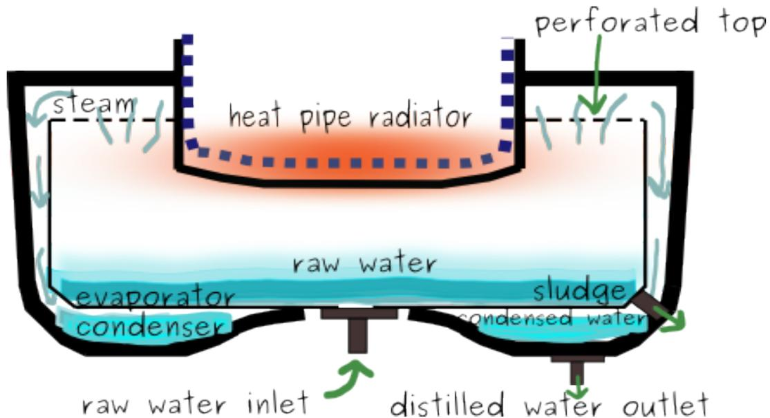
The evaporator-condenser-waster (or sludge) remover is a tightly integrated unit. This is required so that the heat released during condensation may be reused to preheat raw incoming water, which greatly improves the efficiency of the system.
